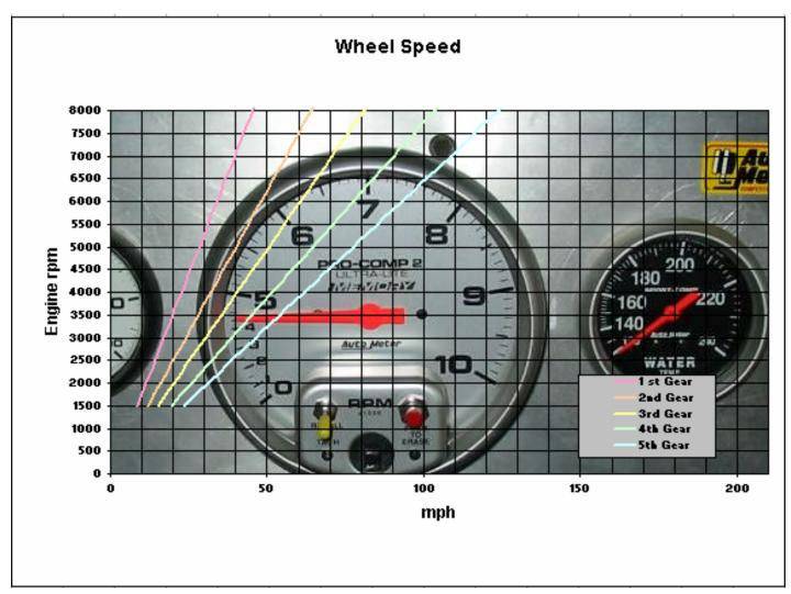
Wheel Speed based on 205 x 50 x 15 Kumho tires at 1841mm circumference and 4.43:1 Final Drive
